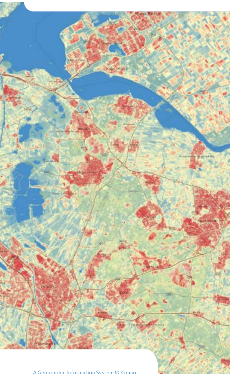
A Geographic Information System (GIS) map. Using available open data we are able to provide clients with relevant area information. This map for example shows heat stress.
